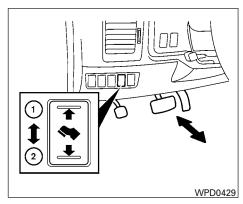
The accelerator and brake pedals can be adjusted for driving comfort.
